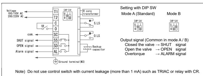
3 way valve: SHUT / Position①, OPEN / Position②
