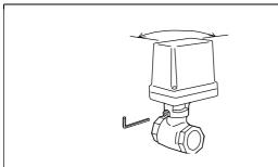
Actuator can be easily removed from the valve by loosing 3 lock screws, and that allows direct operation of the valve.
