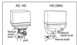
Manual operation can be possible by pulling down manual clutch knob. Set the knob to manual position and operate the joint by using an adjustable wrench in the SHUT/OPEN direction. When it becomes in the position besides the range of operation in the case of manual operation, it may stopped automatic moving.
