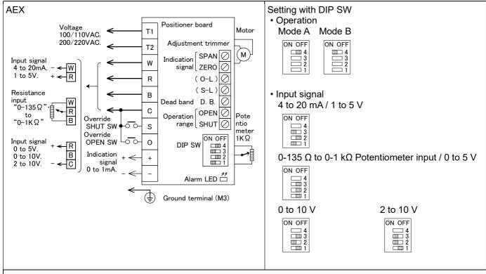
Note • Input signal circuit is non-isolated. Do not connect DC (minus) wire to other DC (minus) common.
