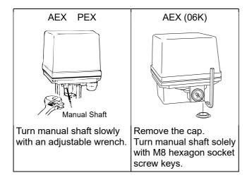
Before automatic operation, be sure to remove the wrench.
