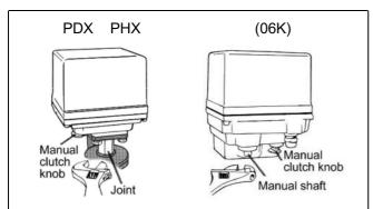
Manual operation can be possible by pulling down manual clutch knob. Set the knob to manual position and operate the joint by using an adjustable wrench in the SHUT/OPEN direction. When it becomes in the position besides the range of operation in the case of manual operation, it may stopped automatic moving.
