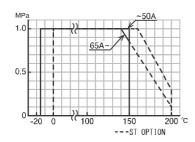
Note) Insulation options are required for use with fluids more than 150 °C.
