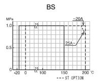
Note) Insulation options are required for use with fluids more than 150 °C.
