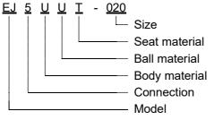
SizeEnter three digits.ex. 20A is 020Seat material①: PTFEBall material①: SUS316 / SCS14ABody material①: SCS14AConnection⑤: Threaded end Rc
