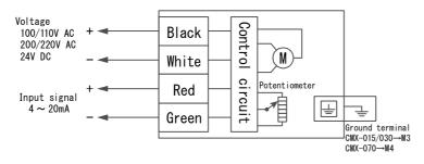
Flexible cable of the actuator has 4 lead wires colored in Black, White, Red, and Green. Check that power supply voltage is correct and connect wires as shown in the wiring diagram.
