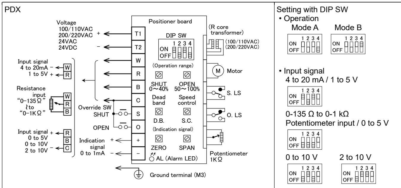
Note) Input signal circuit is non-isolated. Do not connect DC (minus) wire to other DC (minus) common.
