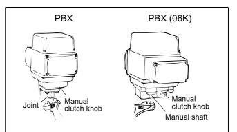
Manual operation can be possible by pulling down manual clutch knob. Set the knob to manual position and operate the joint by using an adjustable wrench in the SHUT/OPEN direction. When it becomes in the position besides the range of operation in the case of manual operation, it may stopped automatic moving. In case the manual clutch knob is not easy to pull down, try moving joint or manual shaft to the opposite direction by wrench. For automatic operation, reset the knob to automatic position.
