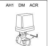
Put an allen wrench (5 mm) or a lever (Φ5.7) into the hole on drive shaft and turn slowly. Manual lever is optional.
