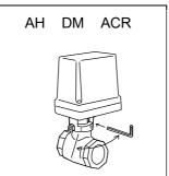
Put an allen wrench (5 mm) or a lever (Φ5.7) into the hole on drive shaft and turn slowly. Manual lever is optional.
