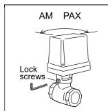
Actuator can be easily removed from the valve by loosing 3 lock screws, and that allows direct operation of the valve. After operation, be sure to put back the actuator to the original position and lock.
